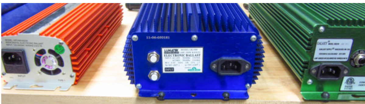
Figure 2 - A close up photo of three typical electronic ballasts.
